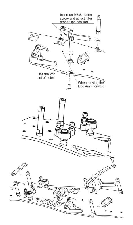
Using 2 x M3x 8 countersunk screw, fix 2 x 26mm post to chassis.
